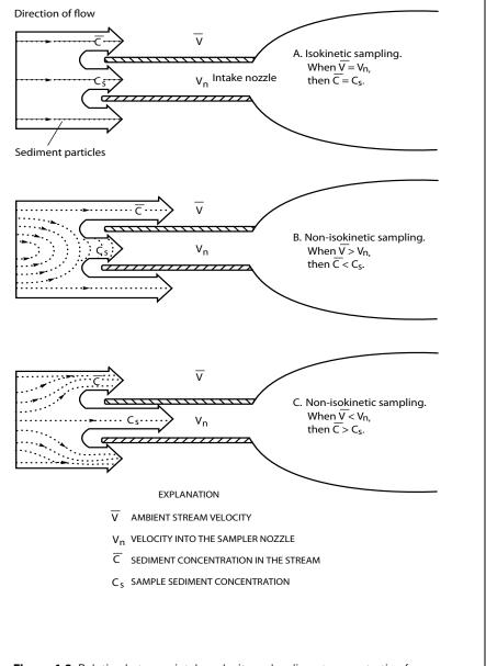
**Figure 4-3.** Relation between intake velocity and sediment concentration for isokinetic and nonisokinetic collection of water samples that contain particulates greater than 0.062 millimeters (modified from Edwards and Glysson, 1999, p. 14).
