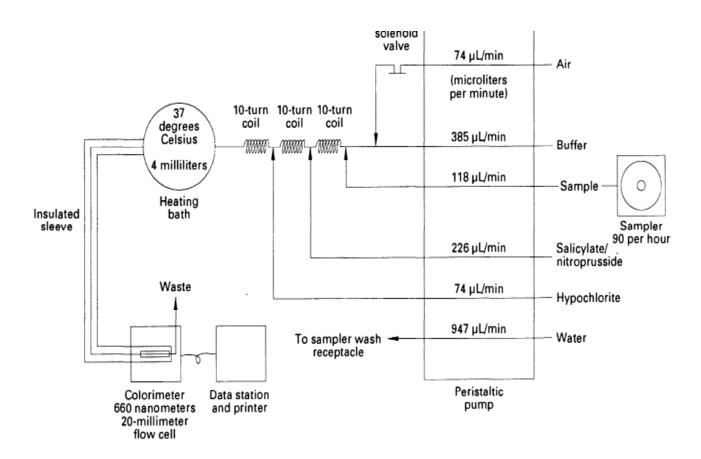
Figure 4.—Nitrogen, ammonia, salicylate-hypochlorite manifold.
