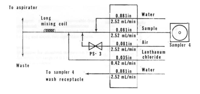
Figure 1. - Magnesium manifold.
