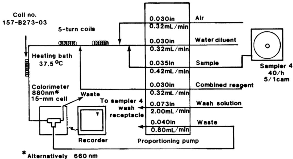
Figure 1. - Phosphorus, phosphomolybdate manifold
