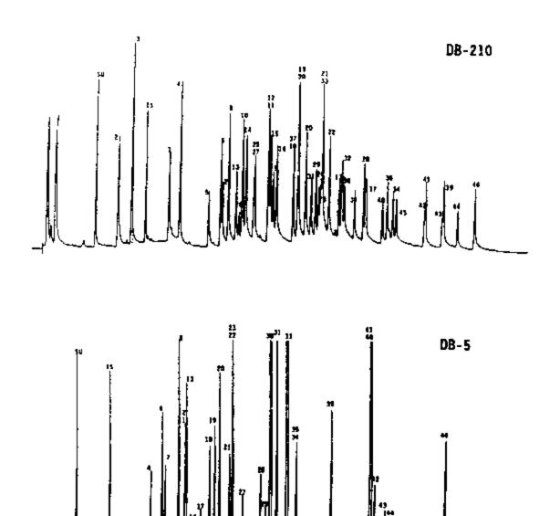
Chromatogram of target organophosphorus compounds on a 30-m DB-5/DB-210 column pair with NPD detector, without simazine, atrazine and carbophenothion. See Table 4 for retention times and for GC operating conditions.
