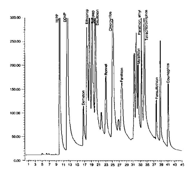
Chromatogram of target organophosphorus compounds from a 15-m DB-210 column with NPD detector. More compounds are shown in Figure 4. See Table 3 for retention times.
