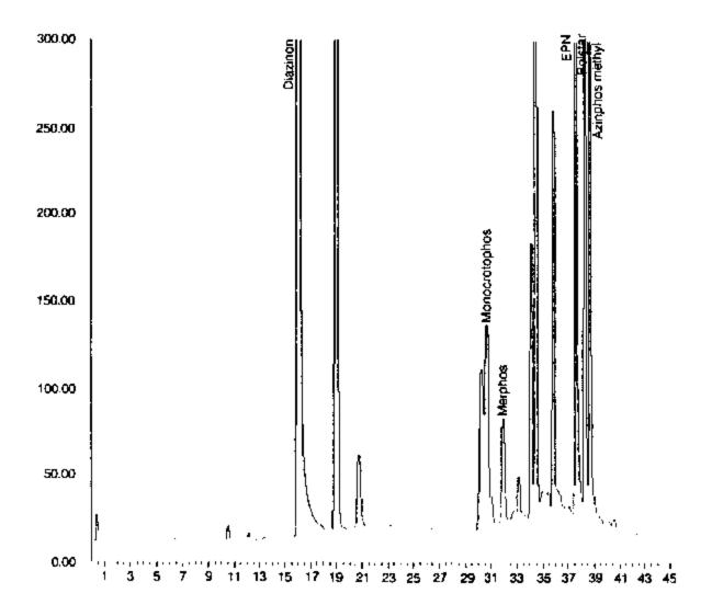
Chromatogram of target organophosphorus compounds from a 15-m DB-210 column with FPD detector. More compounds are shown in Figure 1. See Table 3 for retention times.
