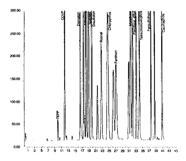
Chromatogram of target organophosphorus compounds from a 15-m DB-210 column with FPD detector. More compounds are shown in Figure 2. See Table 3 for retention times.
