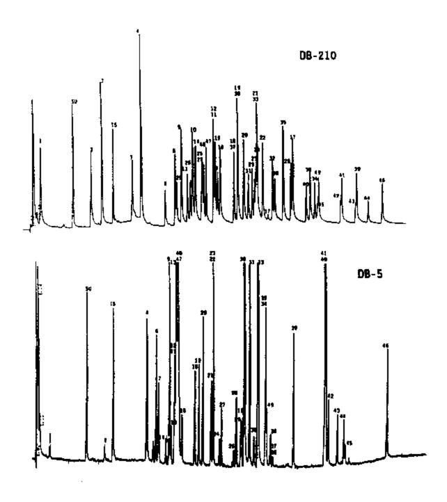
Chromatogram of target organophosphorus compounds on a 30-m DB-5/DB-210 column pair with NPD detector, with simazine, atrazine and carbophenothion. See Table 4 for retention times and for GC operating conditions.
