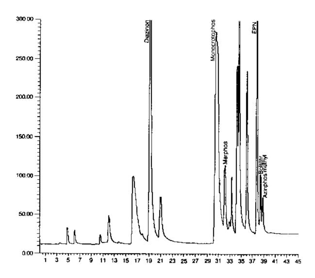
Chromatogram of target organophosphorus compounds from a 15-m DB-210 column with NPD detector. More compounds are shown in Figure 3. See Table 3 for retention times.
